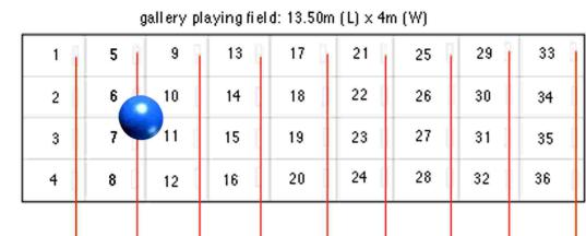
playing field in the gallery is divided into 36 locker units, each 1.5m(L) x 1m(W). each installed a sensor, 36 sensors feed into a sequencer.
